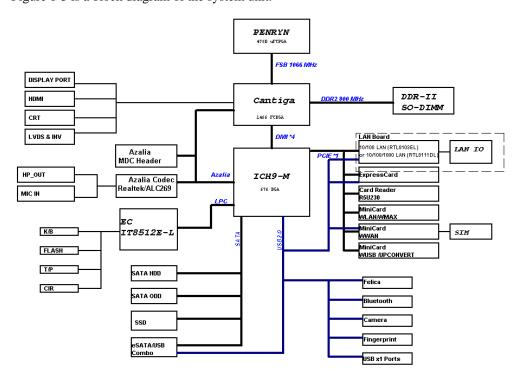
Figure 1-3 System unit block diagram
